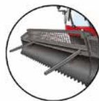
Standard equipment: With the ParkBlade, transporting rails, fun boxes or other park accessories becomes a one-man job.
