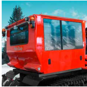
Cab 10 person / 750 kg Cab for moving up to 10 people with 2 foldaway benches.
