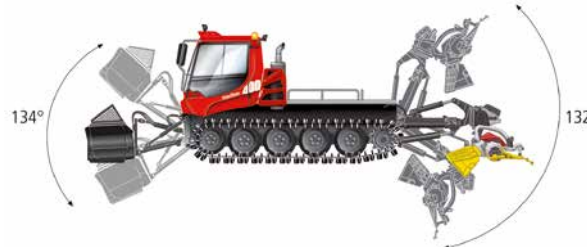
Extreme agility of the front and rear attachments for perfect shaping and reshaping.
