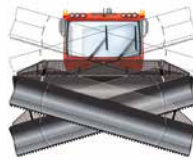
The maximum flexibility of the All-Way-Blade facilitates precise shaping of particular designs.
