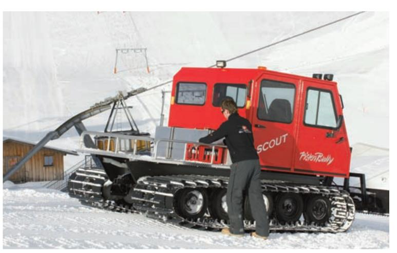
The PistenBully *Scout* platform is as flexible as its area of use is diverse. As a platform for transporting goods it offers enough space and reduces the number of trips required. Work material and tools can also be stored safely.
