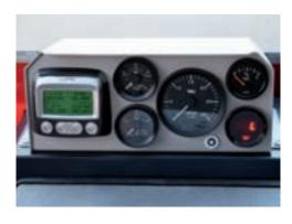
The display instruments on the PistenBully *Scout* are arranged clearly. All important data is available at a glance. The new PowerView Display bundles all information and can be programmed so that the engine switches itself off if preset values are exceeded. For example, this avoids a high revolution speed.
