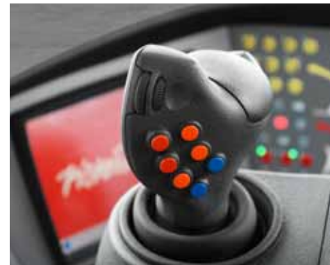
The PistenBully Joystick – all important functions at your fingertips and, thus, quick to access.
