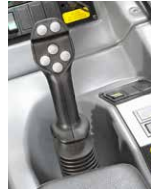
All important functions are integrated into the ergonomically designed joystick.
