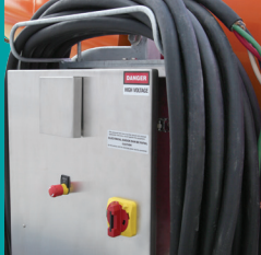
Stainless steel control panel with cord holder
