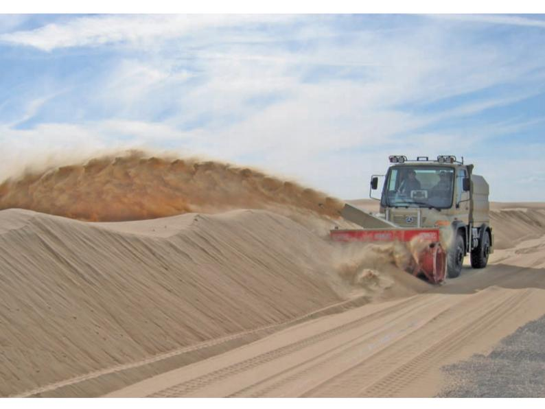
For removing sand from a wide range of road surfaces.
