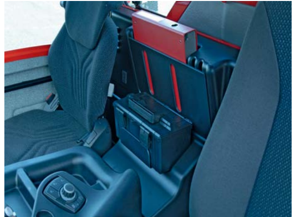
Handy file holder, toolbox and integrated battery and on-board electronic system behind the cover
