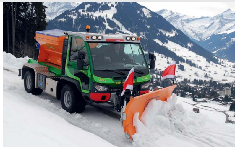
Aebi VT450 Vario snow plough and de-mountable spreader by Schmidt
