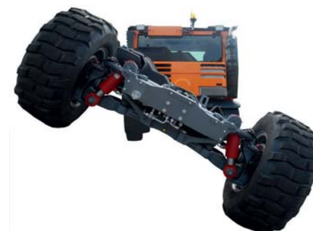
Rear end extremely twisted in relation to the driver's cab (max. \pm 30^\circ )
