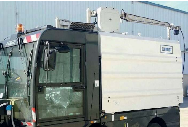
Roof mounted spray boom with a high pressure hand lance
