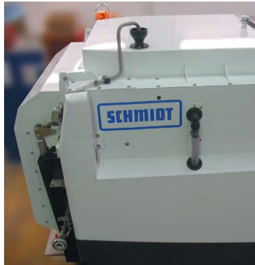
Additional water tank (top)
