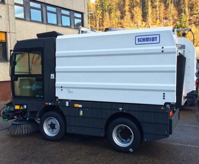
Lateral water tanks
