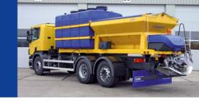
The ACE was developed for the de-icing of airport runways, taxiways and aprons. It applies liquid and solid de-icing agents with extreme accuracy via two special spreading discs. The maximum spraying width is 15 metres and the maximum spreading width 24 metres.
