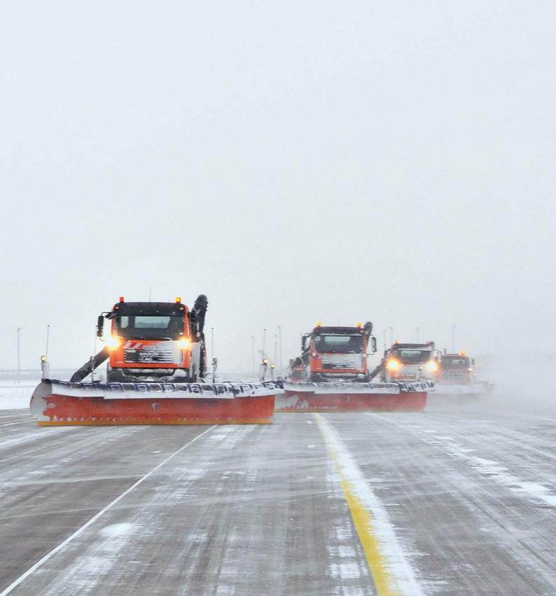
The MS series airport snow ploughs have been specifically developed for the fast and residue-free removal of snow from airport runways, taxiways and airfield aprons. Its innovative obstacle override system enables it to easily overcome surface obstacles, such as concrete irregularities or ground lights.
