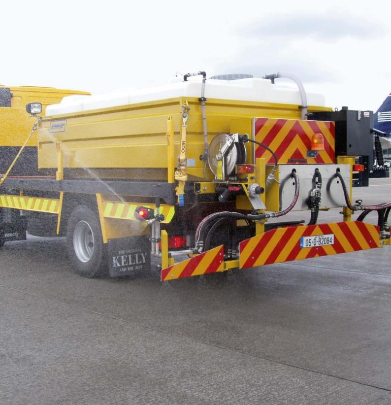
The WSP was developed for the de-icing of airport aprons. Its spray and projection nozzles guarantee highly accurate distribution of the de-icing liquid. The maximum spraying width is 20/24 metres.
