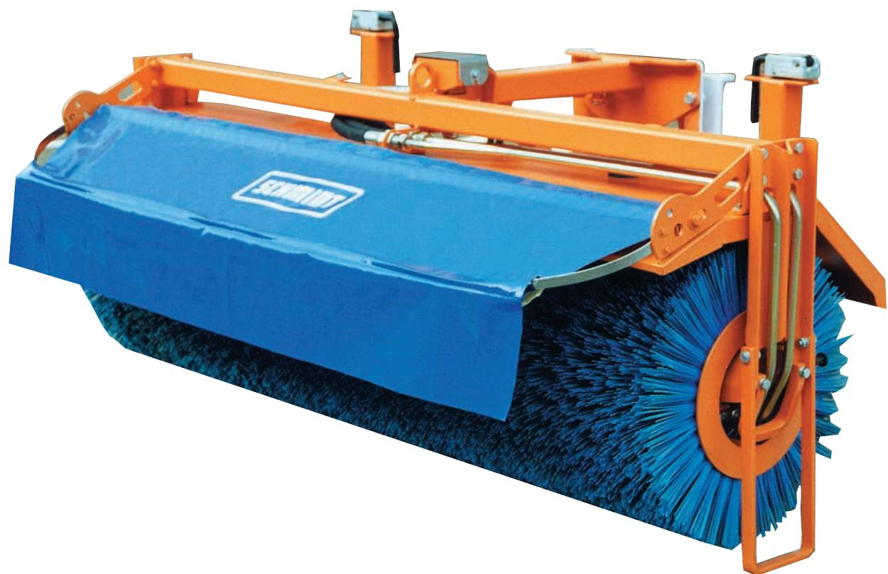
Used with narrow track utility vehicles for cleaning large amounts of heavy dirt.
