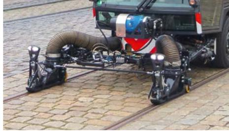
Efficient cleaning of railway tracks embedded in roads is important from both an economic and safety-related point of view. Sand, litter dropped by pedestrians and environmental pollution such as leaves or debris from vehicle tyres can damage the tracks and wheels of trams but also considerably impact upon the stopping distances of these vehicles, and if track grooves are ignored altogether, this can even result in derailment.
