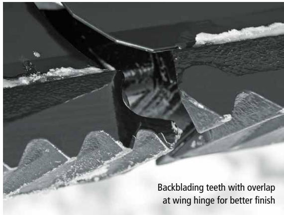
Vertical cutting edge on the wing
