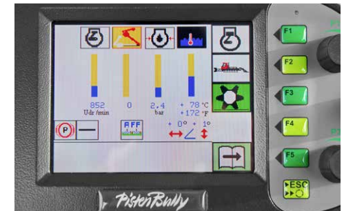
Integrated gradient sensors show the position of the blade and the vehicle in real-time.
