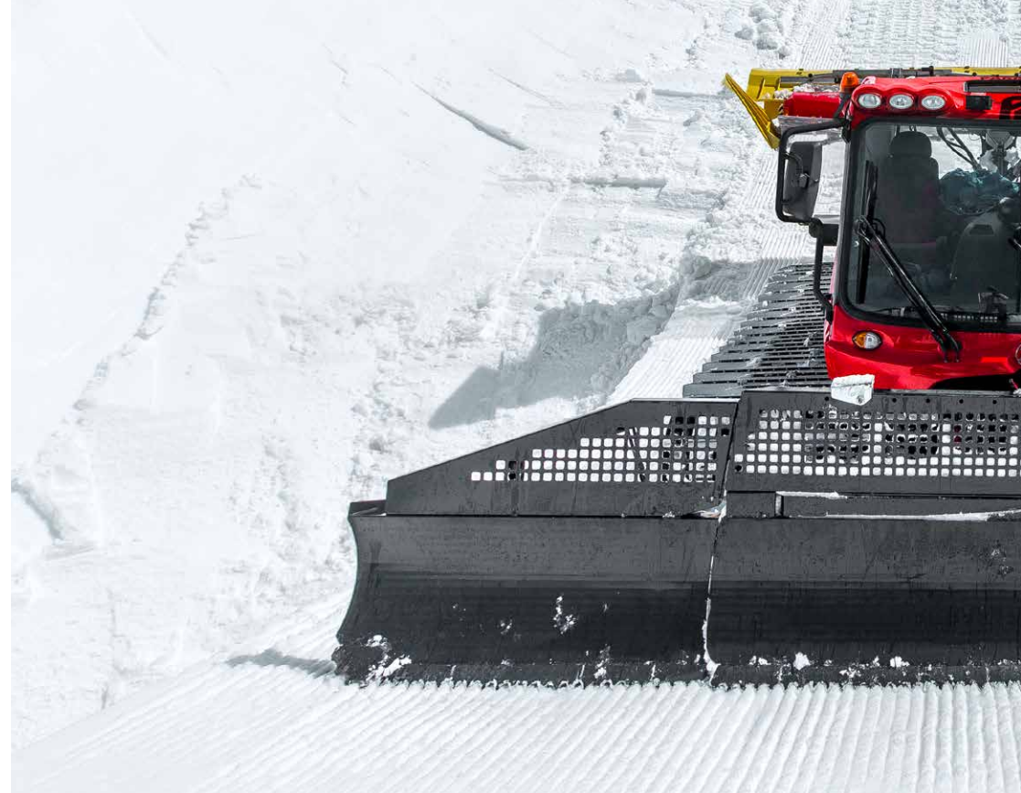
Vertical cutting edge on the wing
