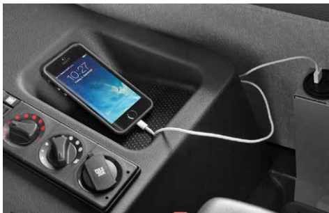
Charger for smartphones, plus USB- and Bluetooth audio connection
