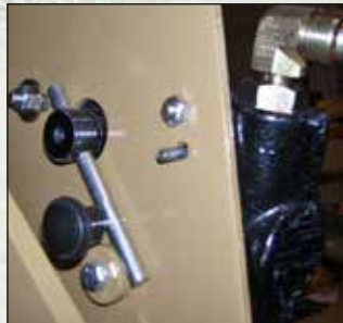
Oscillation control valve - select the exact amount of screen oscillation for varying conditions
