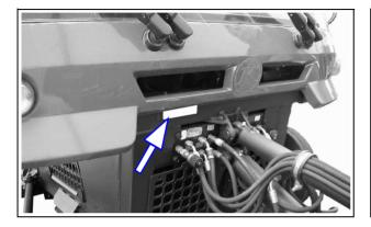
The vehicle number is stamped on the front of the vehicle, on the face end of the right hand frame.
