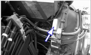
The engine number is stamped on the engine type plate.
