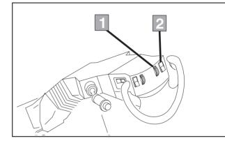
1 Knurled wheel Reducing rotary shaft speed
