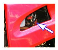
The battery master switch provides a means of isolating the battery from the vehicle's on-board electrics.
