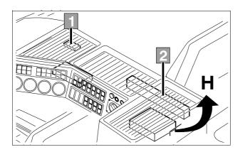
Central console **H** raised by means of recessed grip. Locked by a pneumatic spring support.
