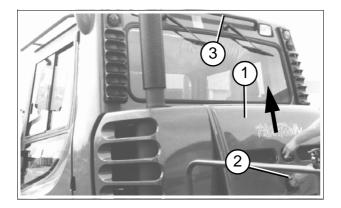
Vehicle batteries are located behind cover 1.
