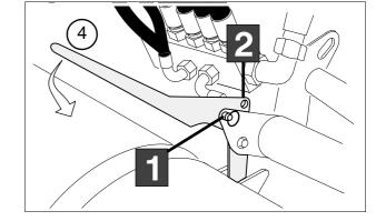
• Actuate pushbutton rotary plough in rigid setting until hydraulic cylinder is completely retracted.
