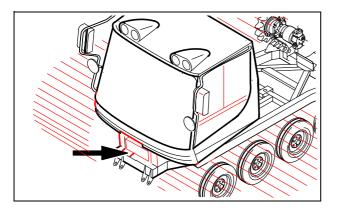
The vehicle identification number (VIN) is embossed on the front of the outside face of the right-hand side of the chassis.
