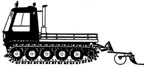
The rear-mounted attachment is an item of auxiliary equipment which should mostly be used with fresh snow and soft spring snow: It packs the snow, smoothes the pistes and obliterates marks left by the tracks. The roller packs the snow in the area between the tracks.
