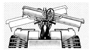
The rotary plough 2000 is hydrostatically driven and is used to loosen up pistes after use by a lot of skiers. It is also used to reduce lumps of snow and ice and to mix up old and fresh snow.
