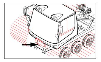
The vehicle identification number (VIN) is embossed on the front of the outside face of the right-hand side of the chassis.
