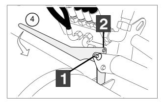
• Actuate pushbutton rotary plough in rigid setting until hydraulic cylinder is completely retracted.
