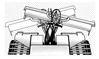
The rotary plough 2000 is hydrostatically driven and is used to loosen up pistes after use by a lot of skiers. It is also used to reduce lumps of snow and ice and to mix up old and fresh snow.
