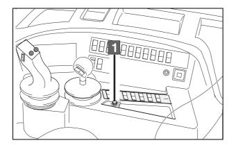
**1 POTENTIOMETER: Downward or loadrelieving pressure on rotary plough** (see Chap. 22/23).
