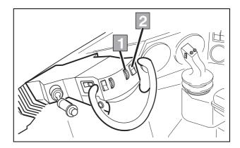
1 KNURLED WHEEL: REDUCTION OF ROTARY PLOUGH SHAFT SPEED.
