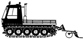
I he rear-mounted attachment is an item of auxiliary equipment which should mostly be used with fresh snow and soft spring snow: It packs the snow, smoothes the pistes and obliterates marks left by the tracks. The roller packs the snow in the area between the tracks.
