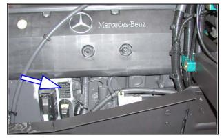
The engine number is embossed on the type plate on the engine.
