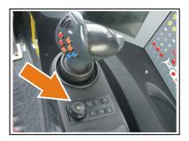
The TCC Terminal Control Centre is an operating unit for the touchscreen in the cockpit. The TCC provides a convenient way of operating the touchscreen while seated. Direct input via the touchscreen itself is not affected, so the two modes can be used in parallel.
