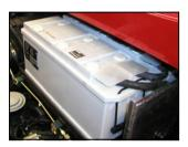
The **two 12 V, 135 Ah/600 A** batteries are mounted on the upper frame.
