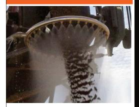
Introduced to address dust issues at conveyor discharge points, the DustBoss Ring creates a curtain around material flow for outstanding particle containment. Engineered for industrial strength and longevity, the DB-R surrounds the discharge flow on all sides, providing simple, focused dust management that's well suited to continuous duty, such as radial stackers.
