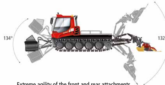
Extreme agility of the front and rear attachments for perfect shaping and reshaping.
