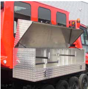
Aluminium ski box Ideal for secure transport of up to 20 pairs of skis or snowboards. Alternatively, you could also store a rescue sledge here. Very easy to fit to the PistonBully.
