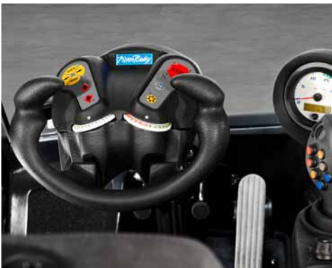
Continuously adjustable – vertically and horizontally – semi-circular steering wheel with multi-function display.
