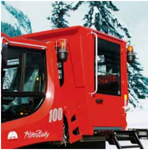
Cab 5 pers. / 700 kg Cab for moving up to 5 people with foldaway bench.
