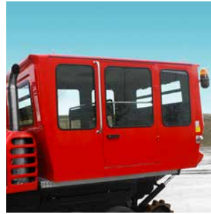
Cab 15 pers. / 1,600 kg Cab for moving up to 15 people with 2 foldaway benches and 2 fixed benches.
