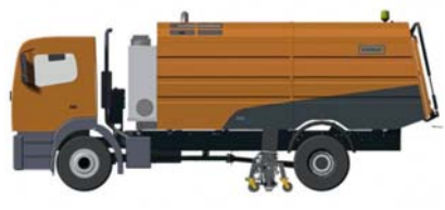
Liquid suction unit (mounted between the axles)
