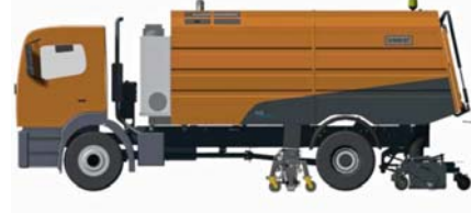
Dual Version: Standard rear mount suction unit (rear mount) and liquid suction unit (mounted between the axles)
