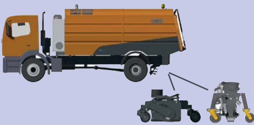
Liquid suction unit (mounted between the axles)
