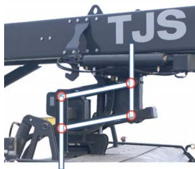
Parallelogram lifting device
