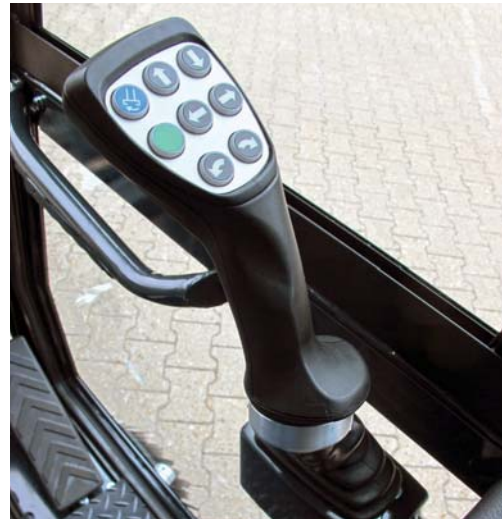
Auto-Drive (operation via control lever)
