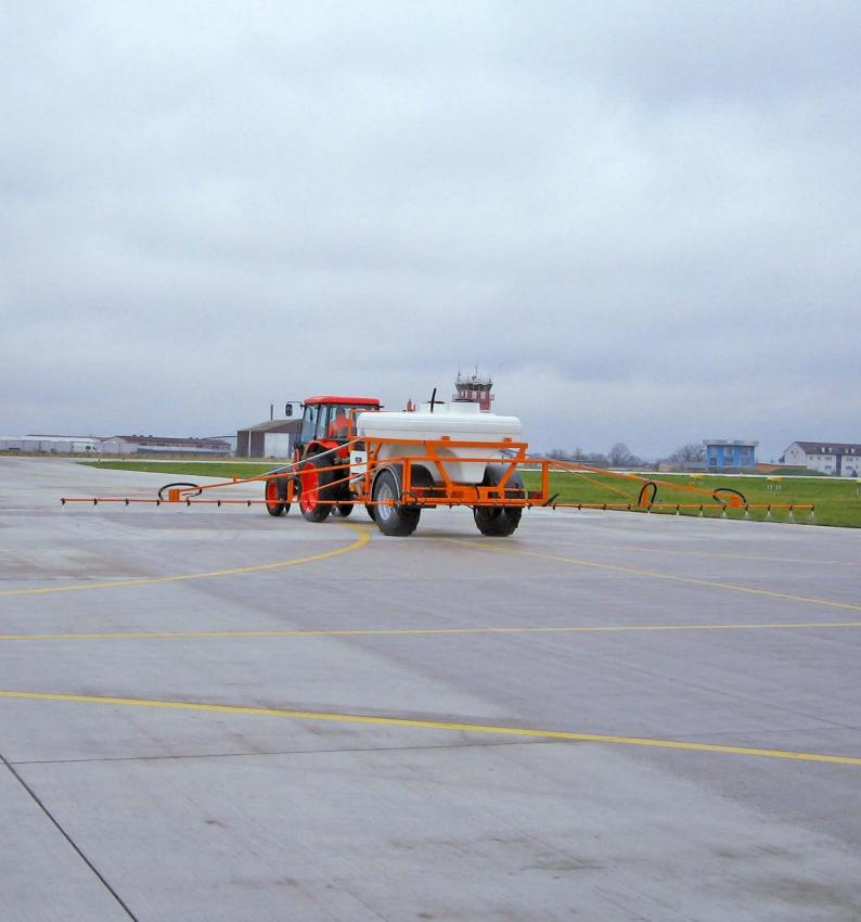
The ASPT is above all ideal for use on the complete airside infrastructure at small airports. The machine delivers de-icer liquid in a very precisely defined dosage via spray nozzles. The trailer-mounted spraying machine can simply be driven from any locally available tractor.
