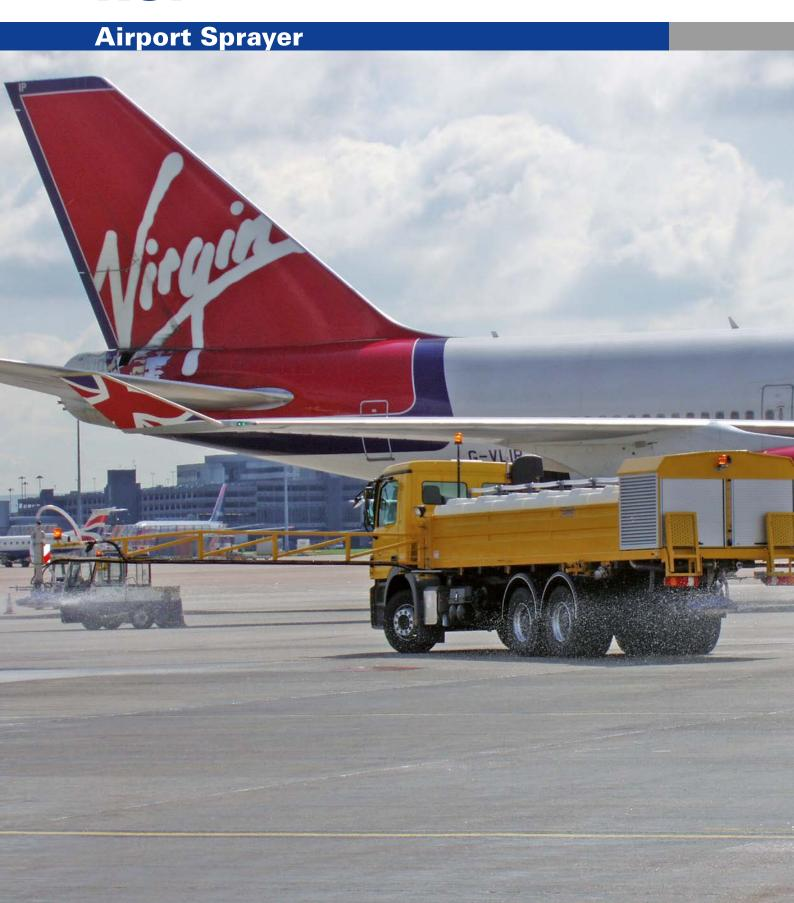
The RSP was developed for de-icing airport runways, taxiways and aprons. It applies de-icing liquids with extreme accuracy via special spraying discs.
