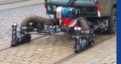
Efficient cleaning of railway tracks embedded in roads is important from both an economic and safety-related point of view. Sand, litter dropped by pedestrians and environmental pollution such as leaves or debris from vehicle tyres can damage the tracks and wheels of trams but also considerably impact upon the stopping distances of these vehicles, and if track grooves are ignored altogether, this can even result in derailment.
