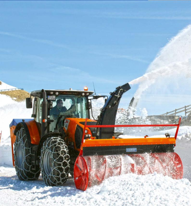
The robust range of FS snow cutter blowers are designed to be mounted on UNIMOGs and tractors and to be used for severe winter municipal road maintenance. They are extremely efficient at clearing high levels of hard, icy snow. They are also capable of removing the side walls of snow left behind by snow ploughs.
