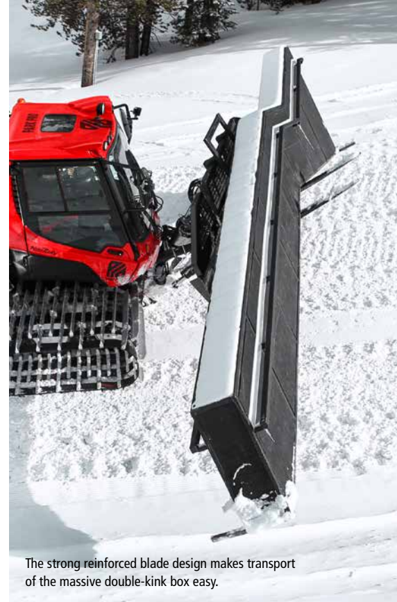
The SwitchBlade 2 is designed to distribute the energy from moving snow evenly across the whole vehicle frame. For maximum stability and thrust.
