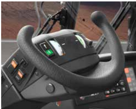
Continuously adjustable semi-circular steering wheel.
