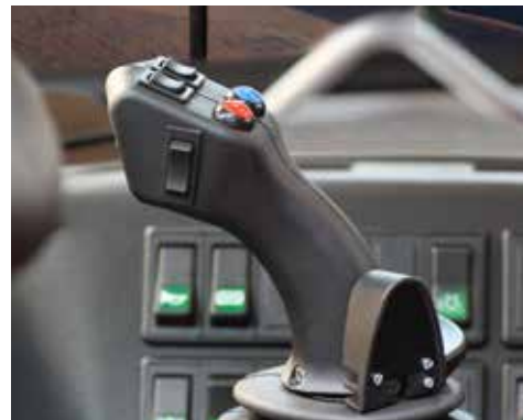
All important functions are integrated into the ergonomically designed joystick.
